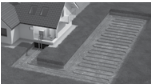
Geothermal Heat Pump System
